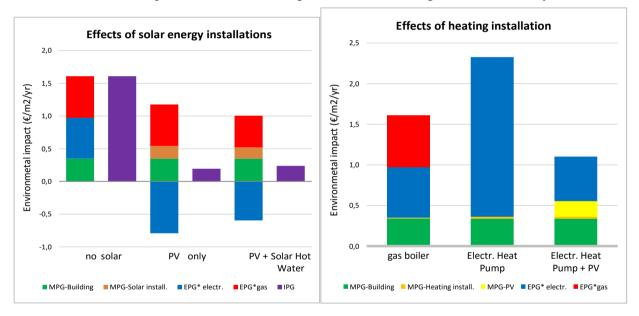
Figure 4: Effects on total environmental impact of building in relation to choice of solar energy installations and choice of the heating installation.
