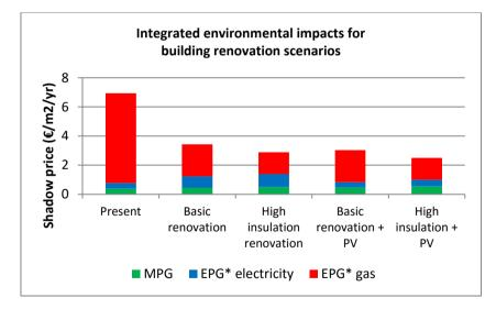
Figure 2: Integrated environmental impacts of building for a number of renovation scenarios. Contributions are shown from materials (MPG), energy consumption gas (EPG\* gas) and energy consumption electricity (EPG\* electricity). Environmental impacts are expressed in shadow price per functional unit according to the Dutch national method for environmental impact assessment of buildings.
